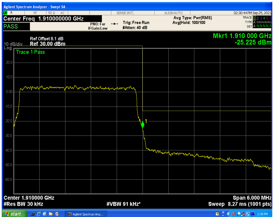
Band2 QAM16 BW=3MHz Channel=19185 RB Size=1 Position=#Max
