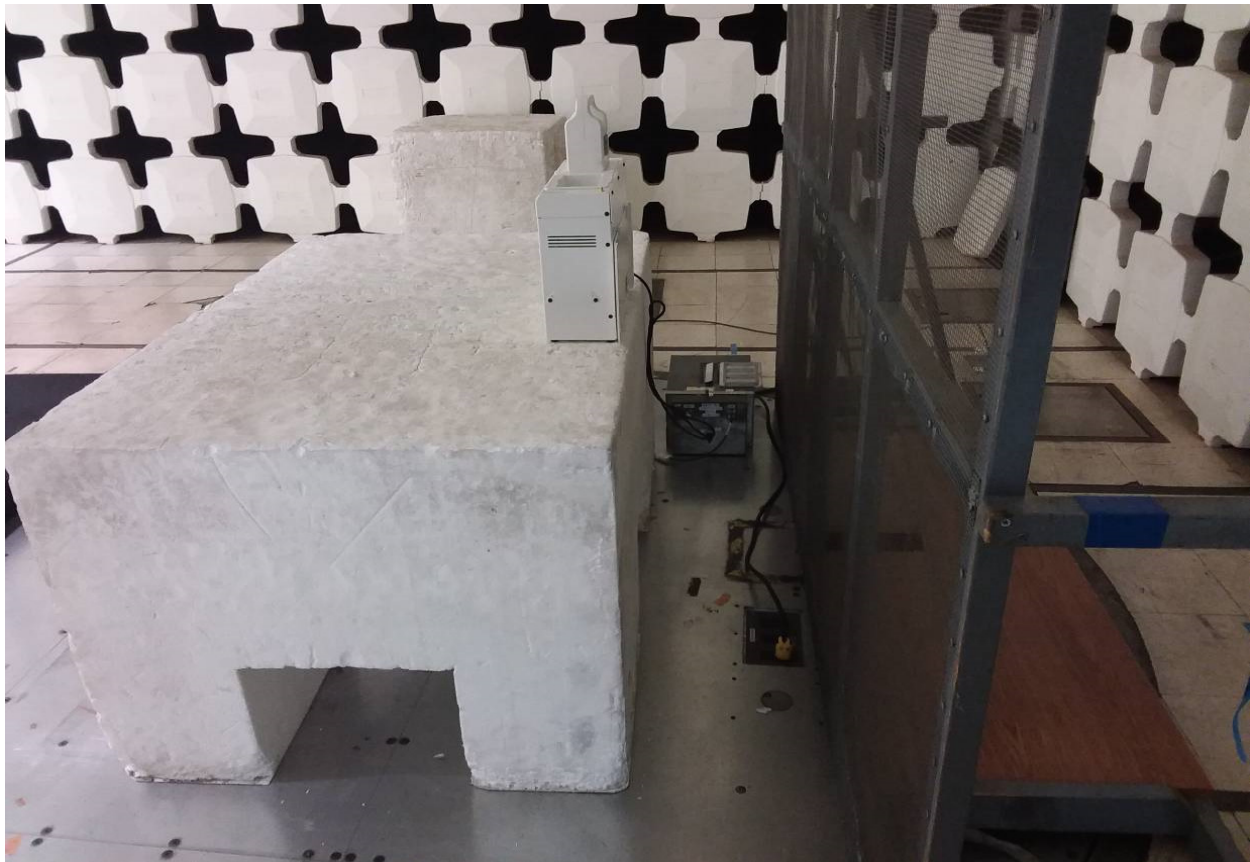
Test Configuration Photograph #2 (Conducted Emissions - Power Port)
