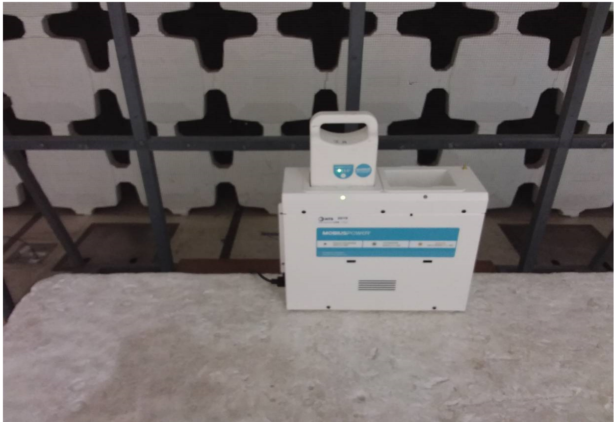
Test Configuration Photograph #1 (Conducted Emissions - Power Port)
