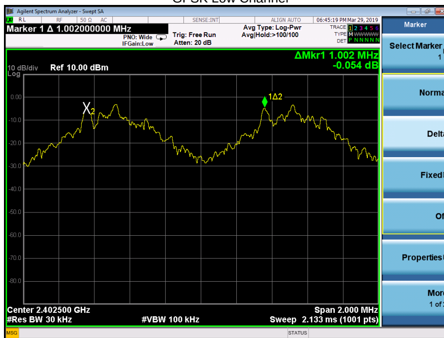
Test plots GFSK Low Channel
