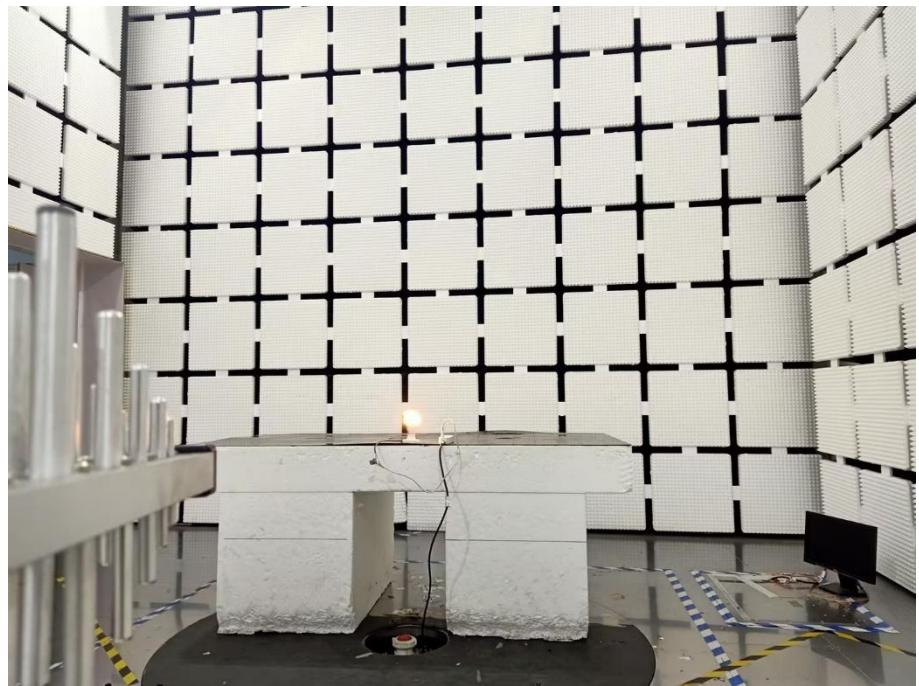
Radiation Emission Test Setup (30MHz to 1GHz)
