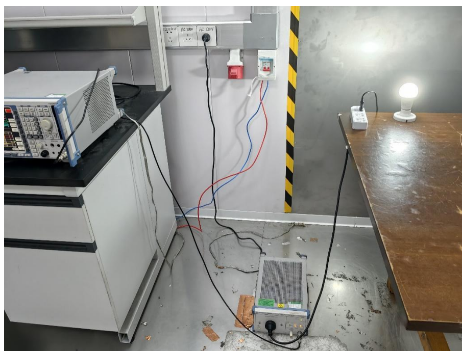
Conducted Emission Test Setup
