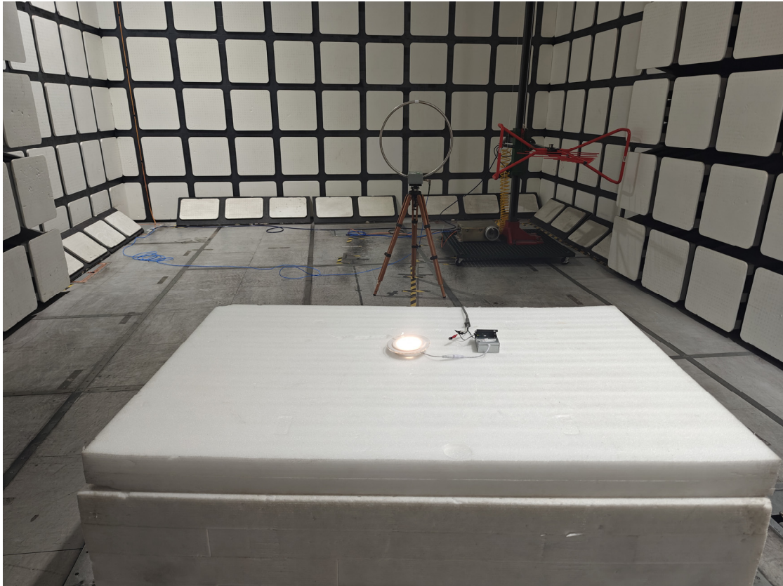
Radiated Emissions View (Below 1 GHz) (Model: H601E)
