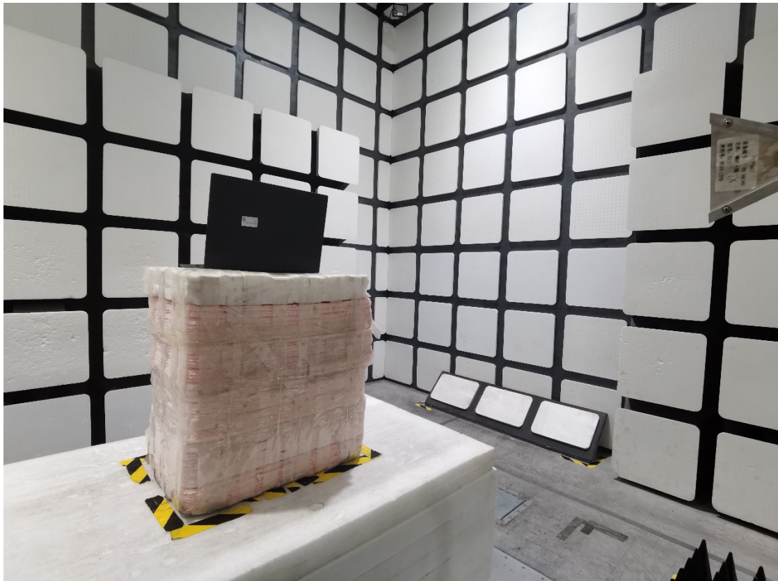
Radiated Emissions View (18-40 GHz)
