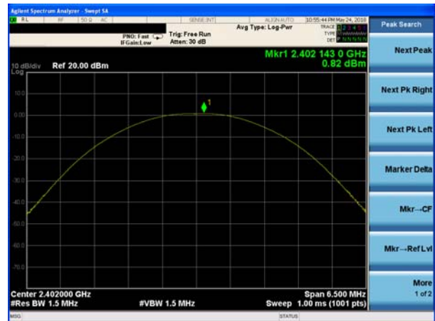
Peak output Power plot on channel 39 (2Mbps)
