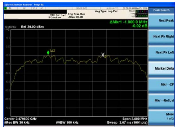
(2Mbps) Channel Separation plot on channel 77-78
