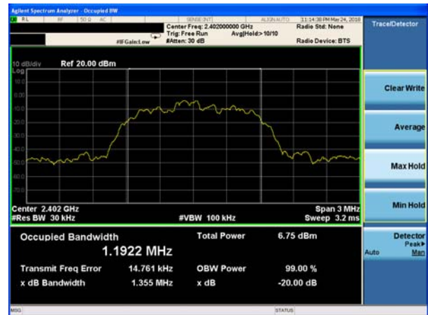
20dB Bandwidth plot on channel 39 (2Mbps)
