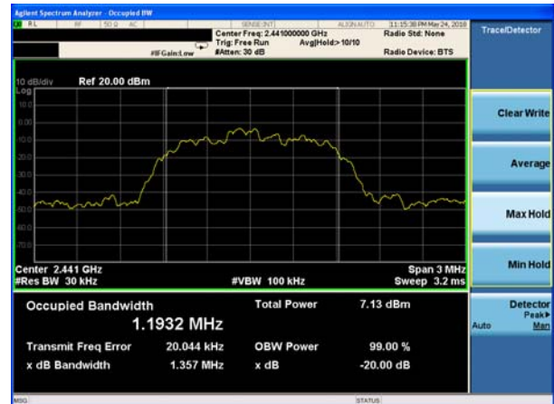
20dB Bandwidth plot on channel 78 (2Mbps)
