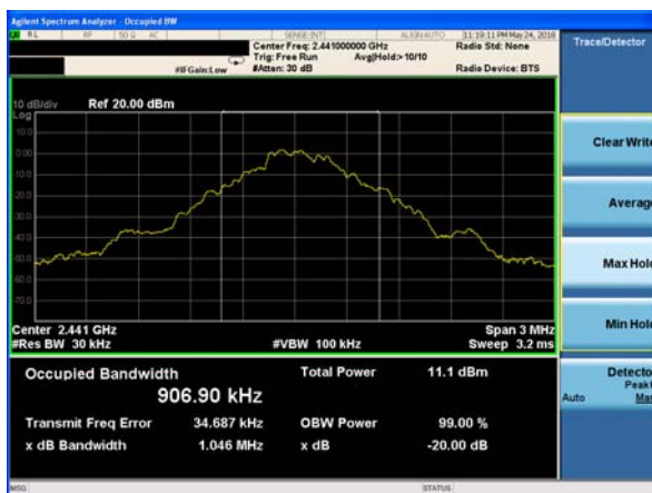
20dB Bandwidth plot on channel 78 (1Mbps)
