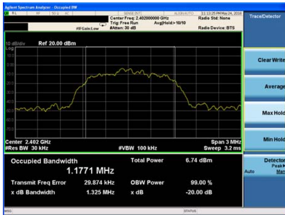
20dB Bandwidth plot on channel 39 (3Mbps)
