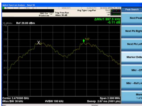
(1Mbps) Channel Separation plot on channel 77-78
