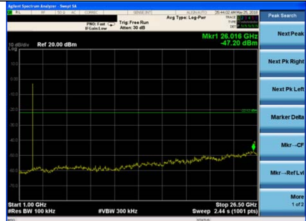
GFSK on channel 78
