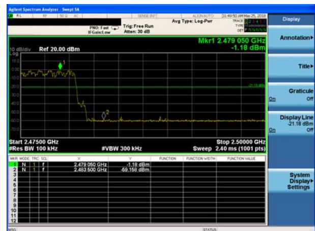
8-DPSK: Band Edge-High Channel (Hopping Mode)
