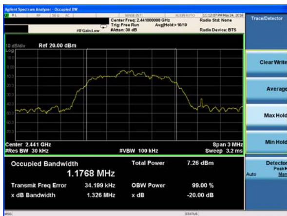
20dB Bandwidth plot on channel 78 (3Mbps)
