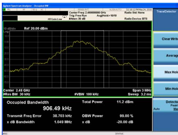
20dB Bandwidth plot on channel 78 (1Mbps)
