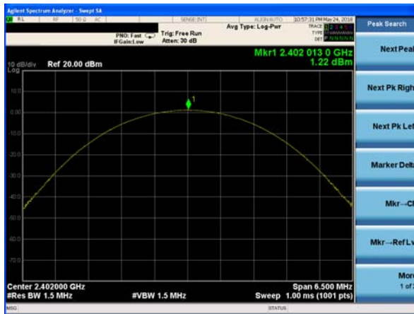
Peak output Power plot on channel 39 (3Mbps)
