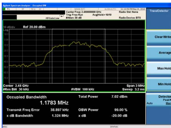
20dB Bandwidth plot on channel 78 (3Mbps)
