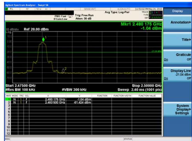
\pi /4-DQPSK: Band Edge-High Channel (Hopping Mode)
