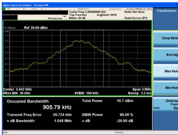
20dB Bandwidth plot on channel 39 (1Mbps)
