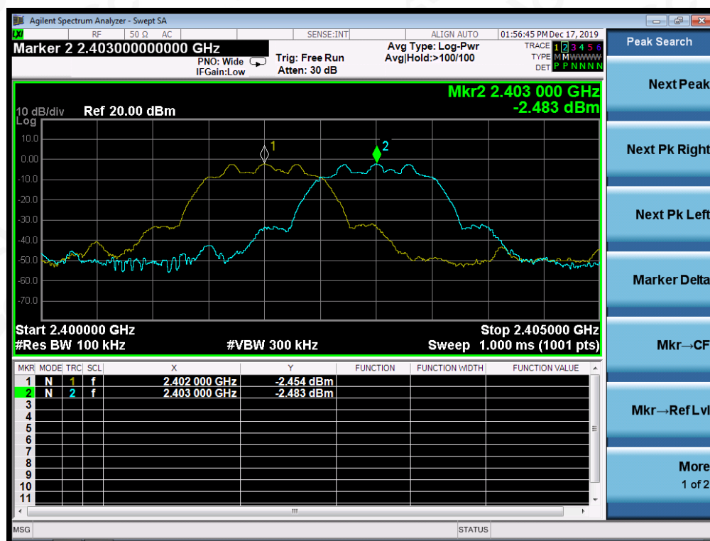
TEST PLOT FOR FREQUENCY SEPARATION
