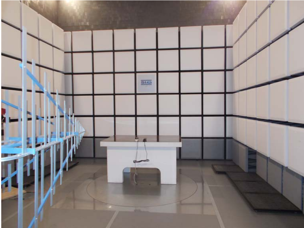
Figure 4: Radiated emission test – 200 MHz – 1000 MHz (with charger)
