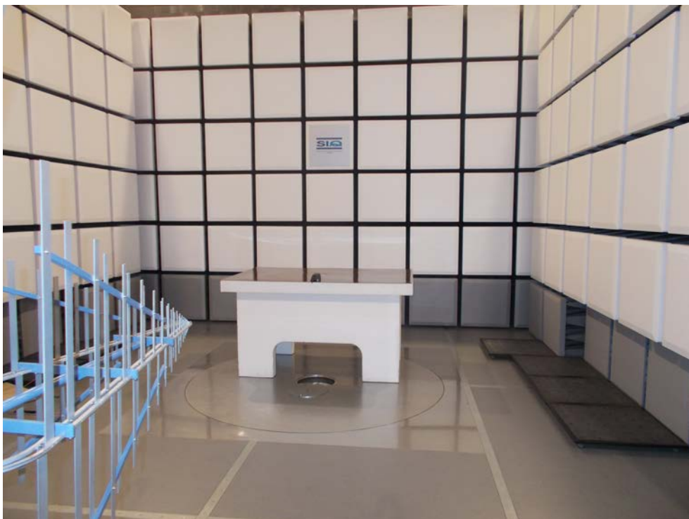
Figure 5: Radiated emission test – 200 MHz – 1000 MHz (without charger)
