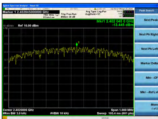
GFSK (BLE 1Mbps) LOW CHANNEL
