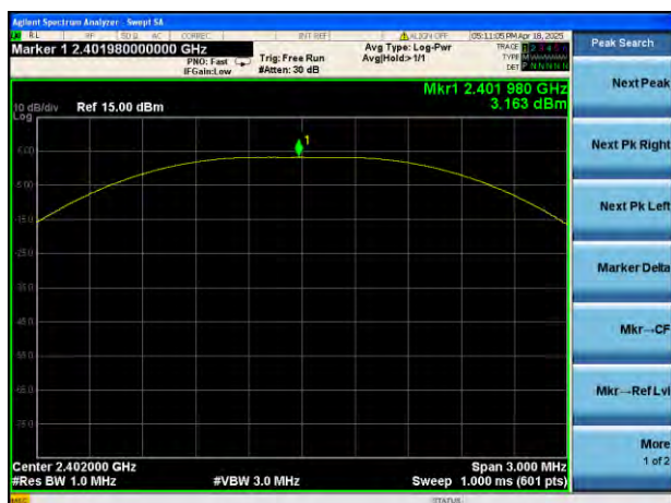
GFSK (BLE 1Mbps) LOW CHANNEL
