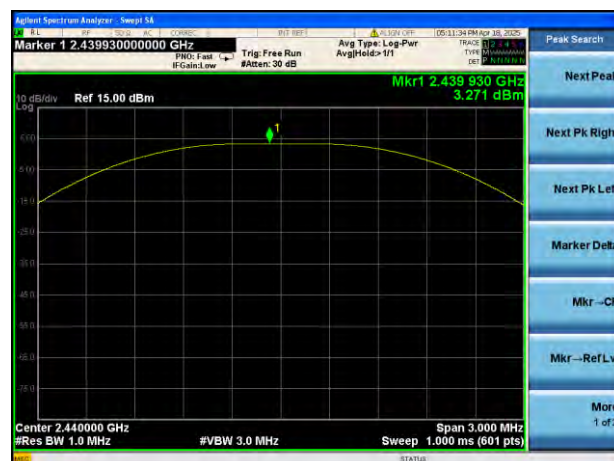
GFSK (BLE 1Mbps) MIDDLE CHANNEL
