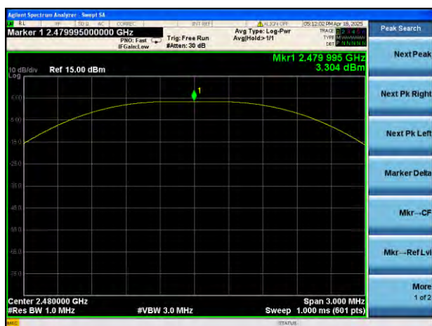
GFSK (BLE 1Mbps) HIGH CHANNEL
