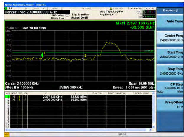
GFSK LOW CHANNEL, BAND EDGE
