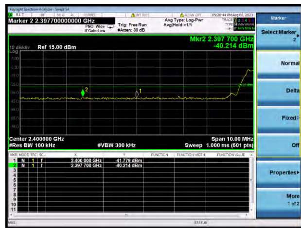
GFSK LOW CHANNEL, BAND EDGE
