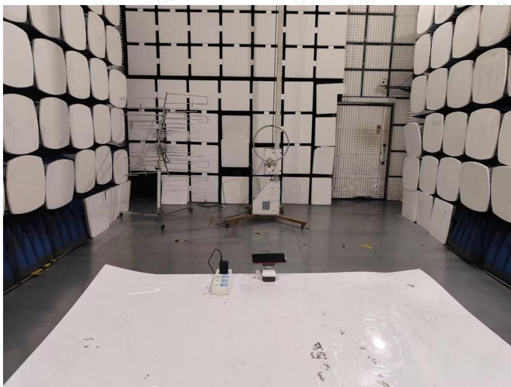
Radiated Emission below 30MHz-AC adapter charge mode
