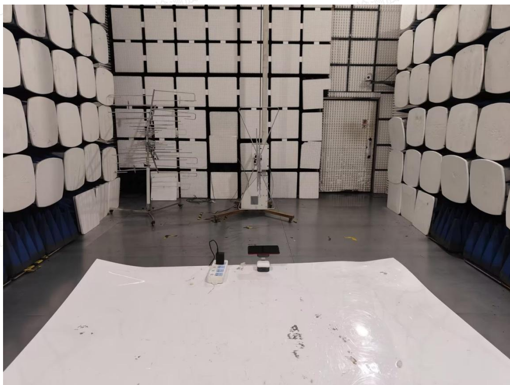
Radiated Emission below 1GHz-AC adapter charge mode
