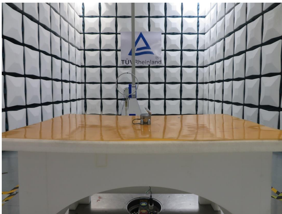
Photograph 2: Set-up photo for Radiated Emission, Below 30MHz
