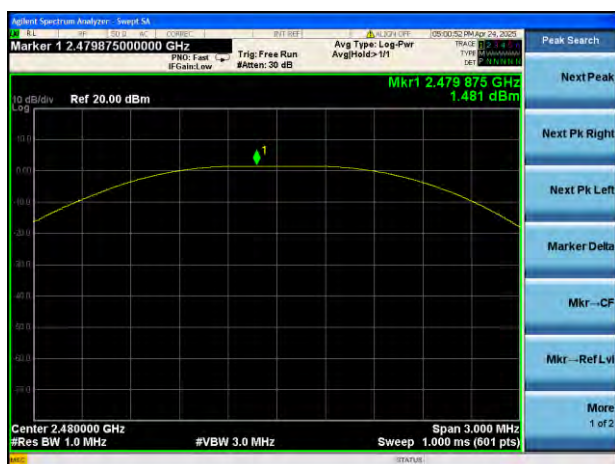
GFSK (BLE 1Mbps) HIGH CHANNEL
