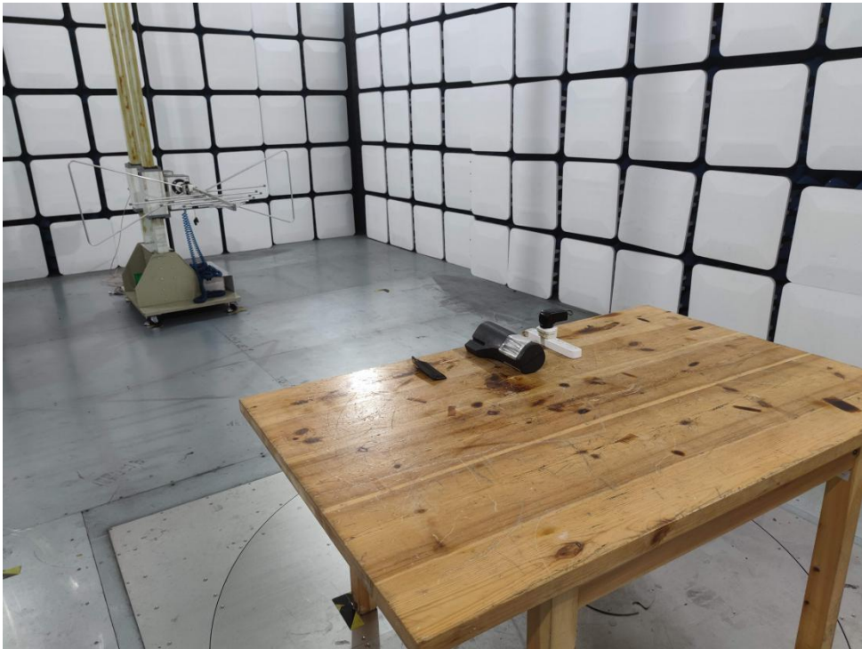
Photo of Radiation Emission Test
