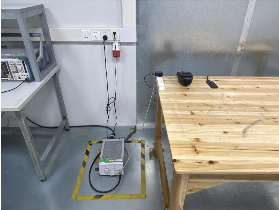
Photo of Conducted Emission Measurement
