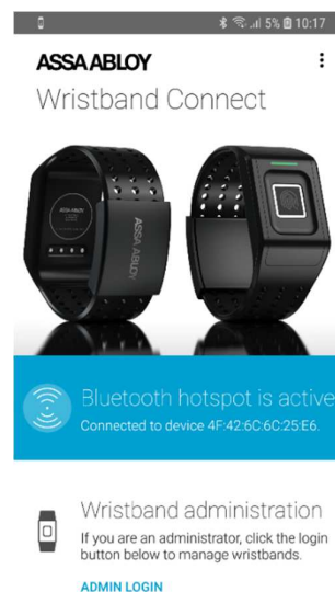
Figure 2: The Wristband Connect app establishes a Bluetooth hotspot for the Wristband's communication with the Service Backend.
