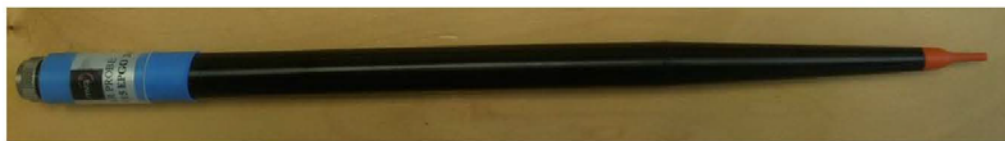
Figure 1 – MVG COMOSAR Dosimetric E field Dipole
