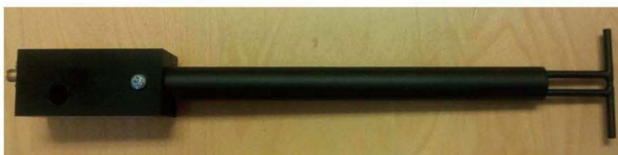
Figure 1 – MVG COMOSAR Validation Dipole
