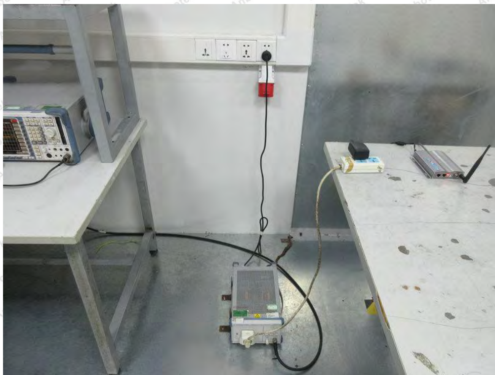
Photo of Conducted Emission Measurement
