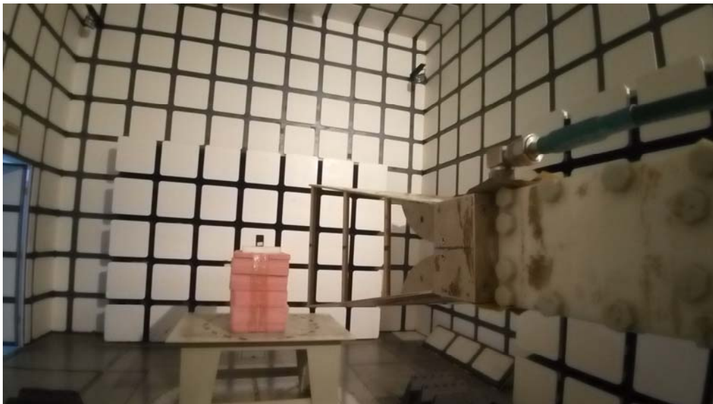
Radiated Emissions View (Above 1 GHz)
