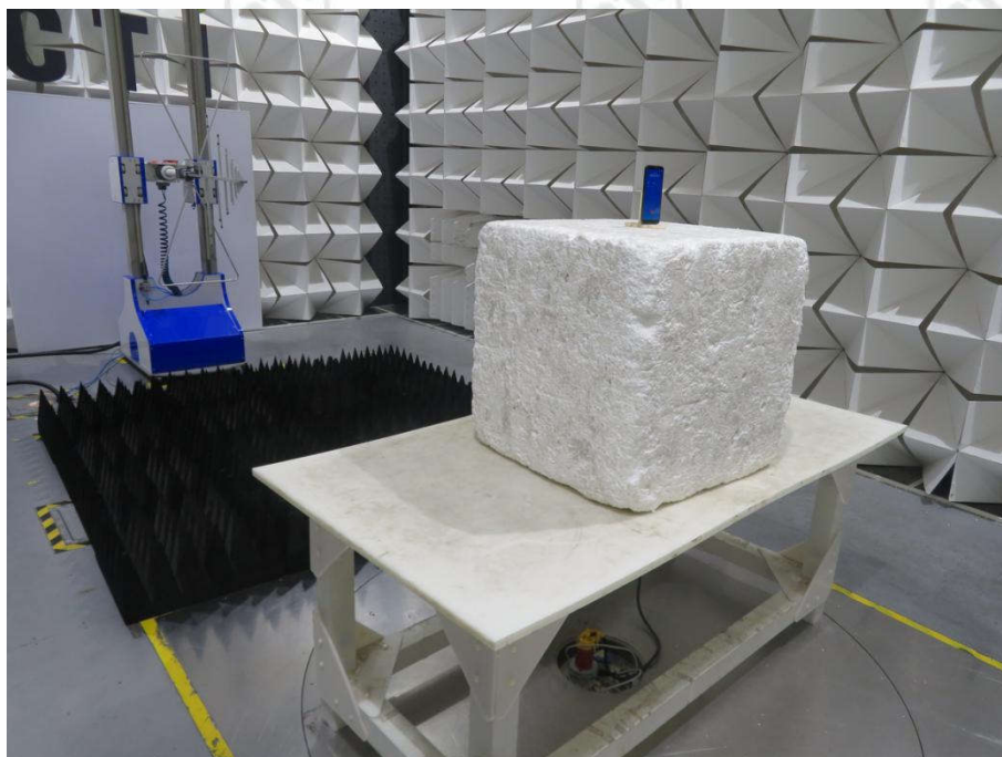
Radiated spurious emission Test Setup-1(Below 1GHz)
