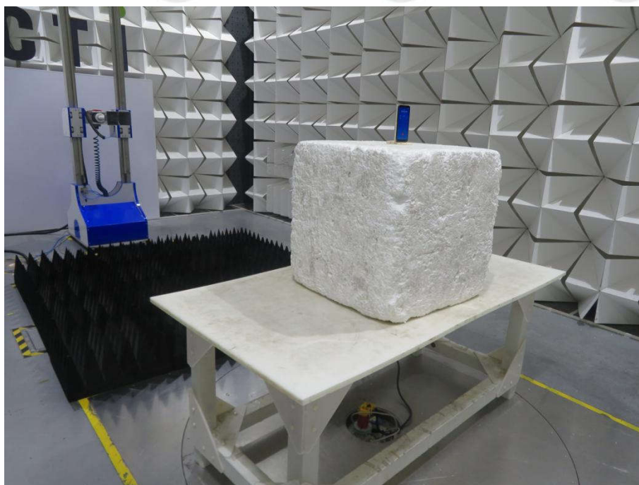
Radiated spurious emission Test Setup-2(Above 1GHz)
