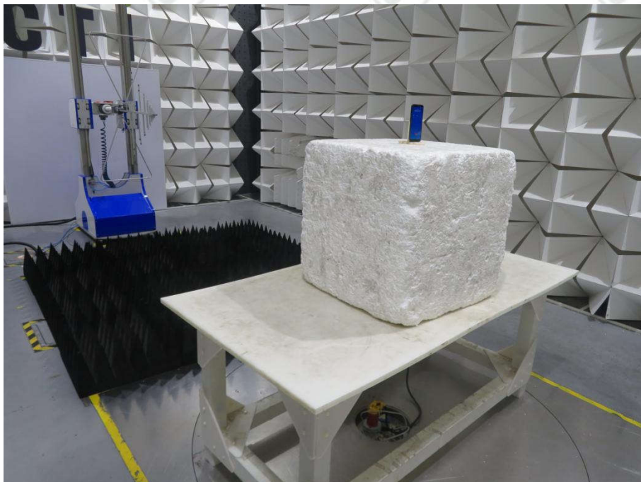
Radiated spurious emission Test Setup-1(Below 1GHz)
