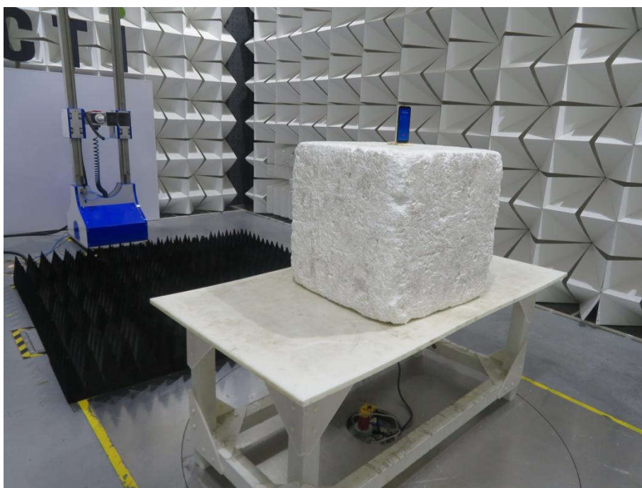
Radiated spurious emission Test Setup-2(Above 1GHz)
