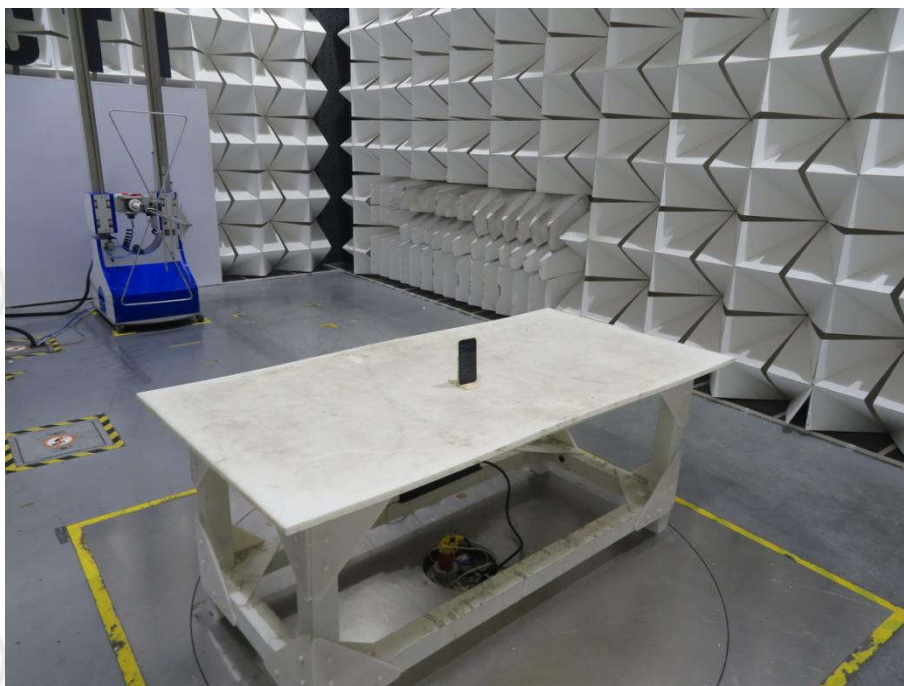
Radiated spurious emission Test Setup-1(Below 1GHz)
