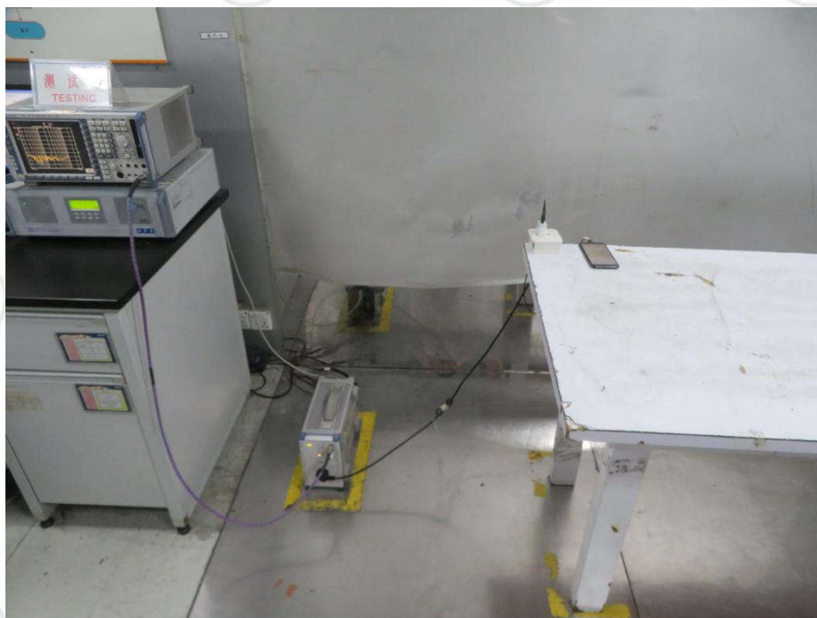
Conducted Emissions Test Setup
