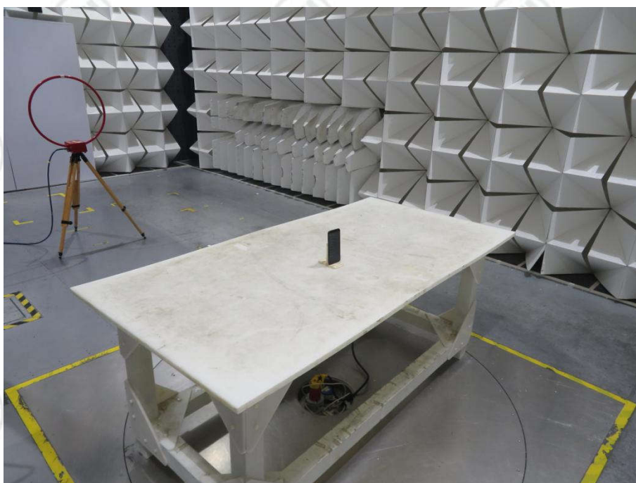
Radiated spurious emission Test Setup-2(Below 30M)
