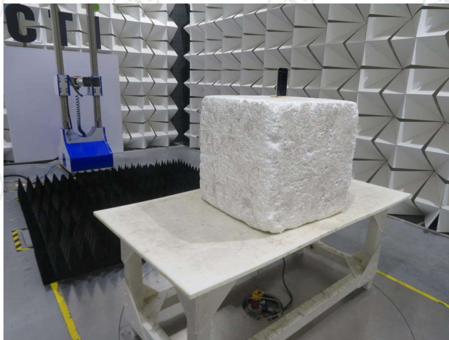
Radiated spurious emission Test Setup-3(Above 1GHz)
