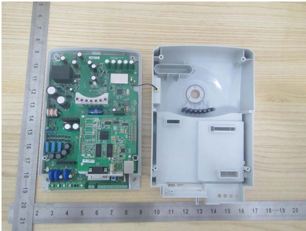
Internal View of EUT-3
