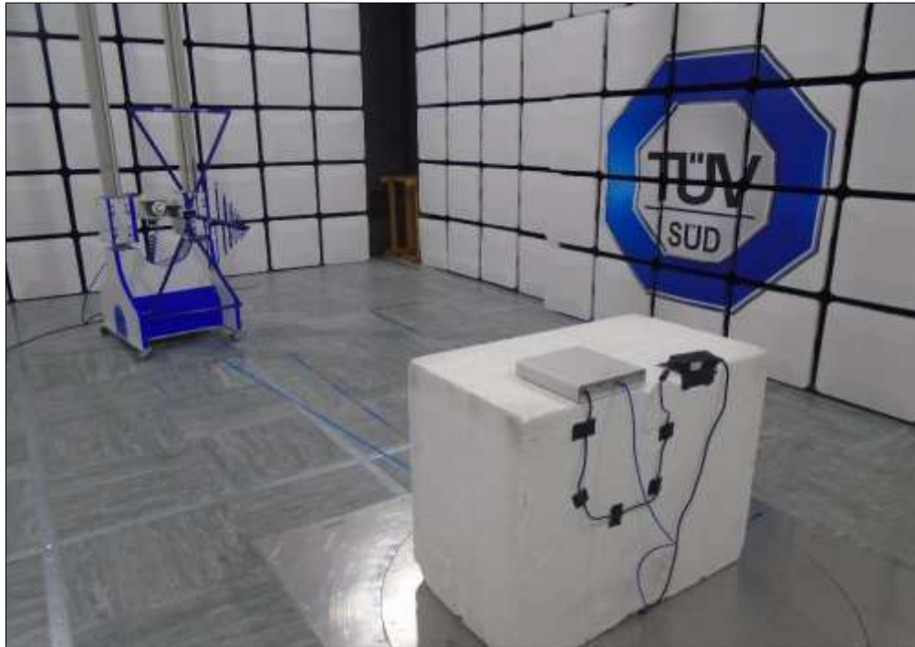
Figure 12 - Test Setup - Below 1 GHz
