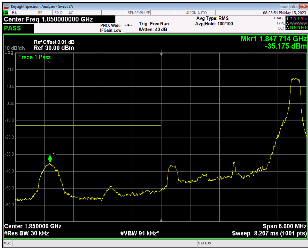
Band2 QPSK BW=3MHz Channel=18615 RB Size=15 Position=#0
