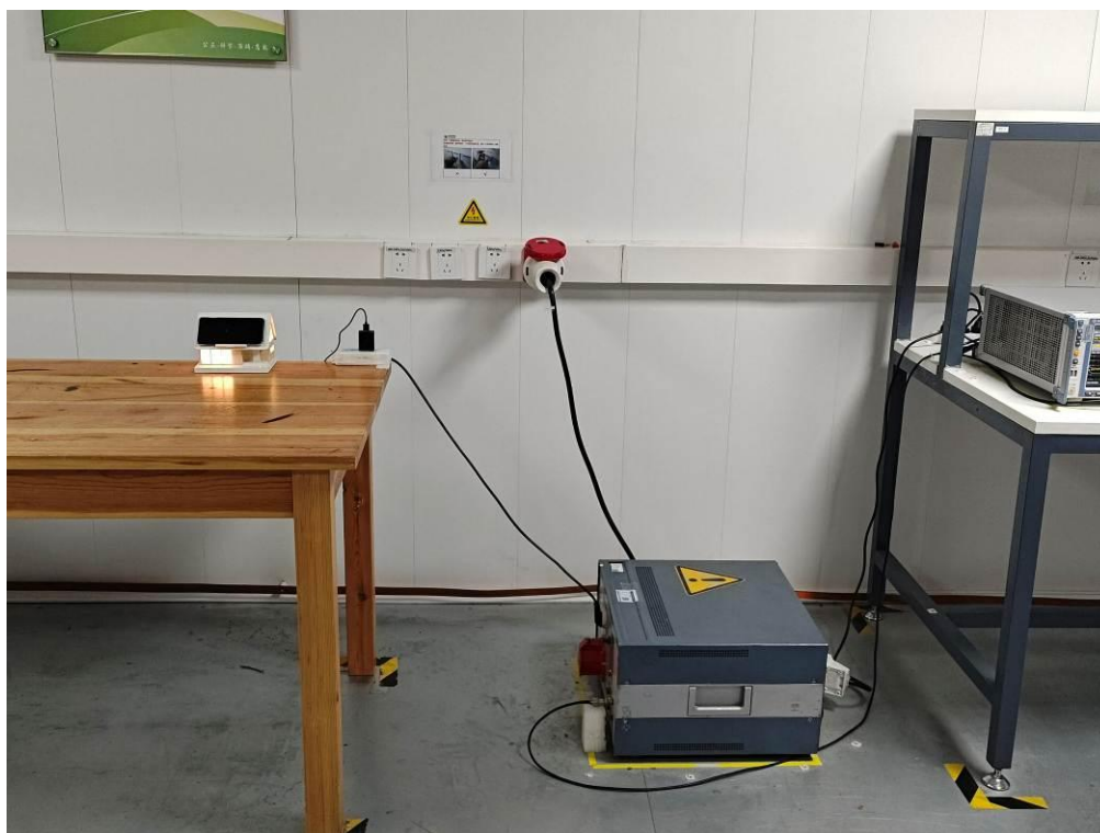
Conducted Emission-AC adapter charge mode
