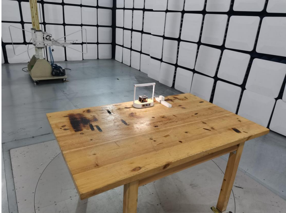
Photo of Radiation Emission Test
