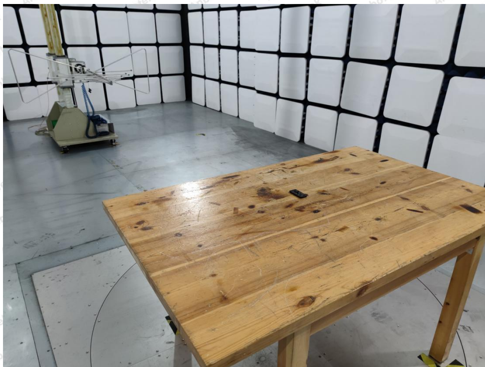
Photo of Radiation Emission Test
