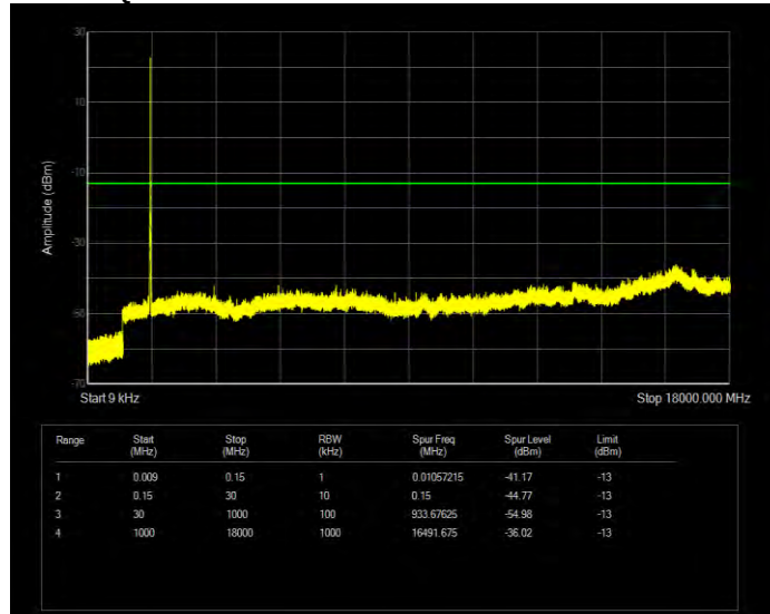
Band71 16QAM BW=10MHz Channel=133172 RB Size=50 Position=#0
