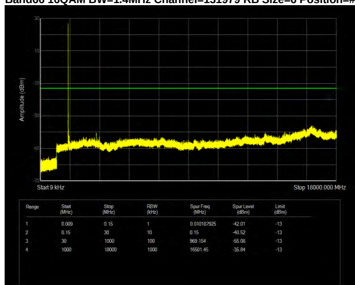
Band66 16QAM BW=1.4MHz Channel=131979 RB Size=6 Position=#0
