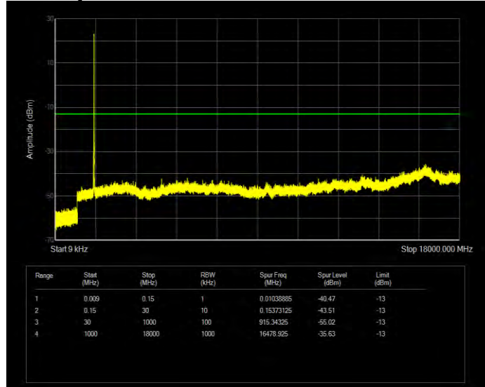
Band66 QPSK BW=5MHz Channel=132647 RB Size=25 Position=#0
