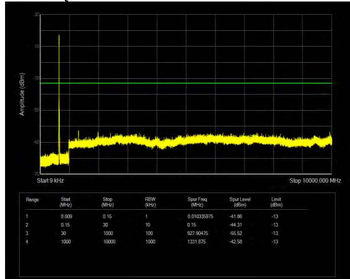
Band71 16QAM BW=5MHz Channel=133147 RB Size=25 Position=#0
