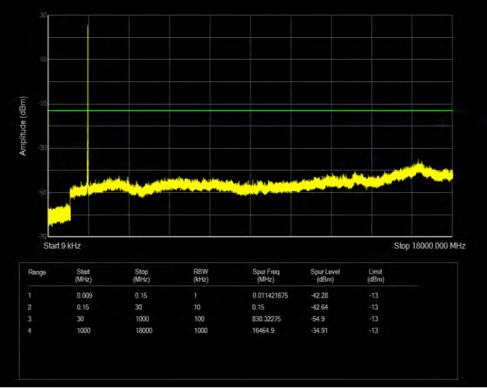
Band66 16QAM BW=5MHz Channel=131997 RB Size=25 Position=#0
