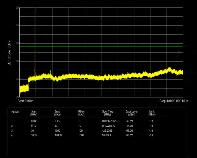
Band66 QPSK BW=1.4MHz Channel=131979 RB Size=6 Position=#0
