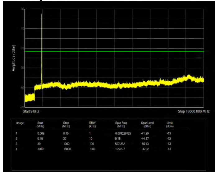
Band66 16QAM BW=3MHz Channel=131987 RB Size=15 Position=#0
