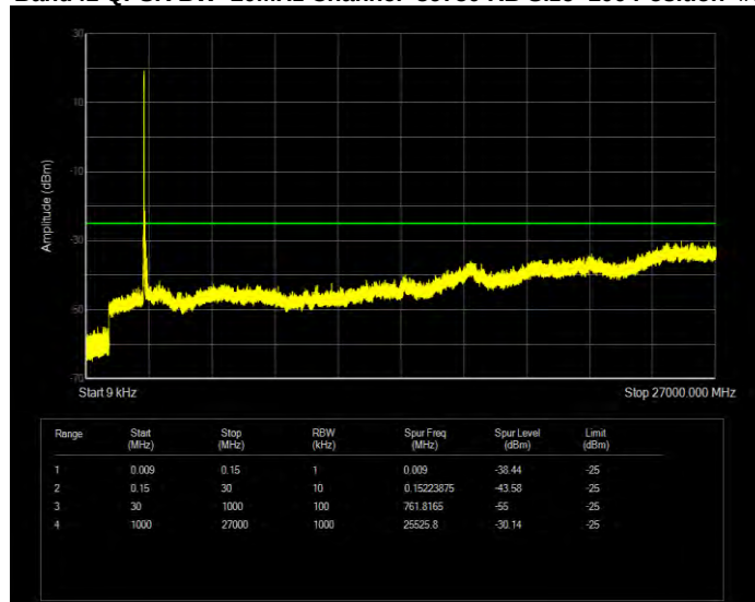
Band41 QPSK BW=20MHz Channel=39750 RB Size=100 Position=#0
