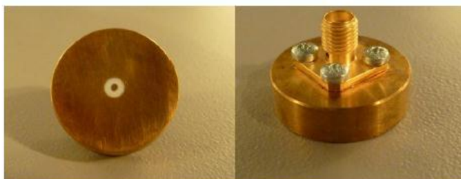
Figure 1 – MVG LIMESAR Dielectric Probe
