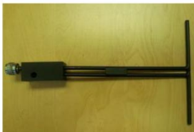
Figure 1 – MVG COMOSAR Validation Dipole
