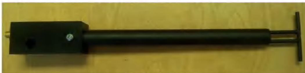
Figure 1 – MVG COMOSAR Validation Dipole
