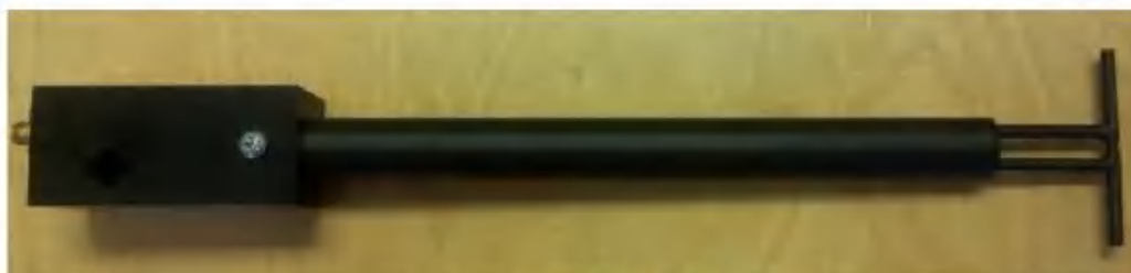
Figure 1 – MVG COMOSAR Validation Dipole
