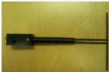
Figure 1 – MVG COMOSAR Validation Dipole
