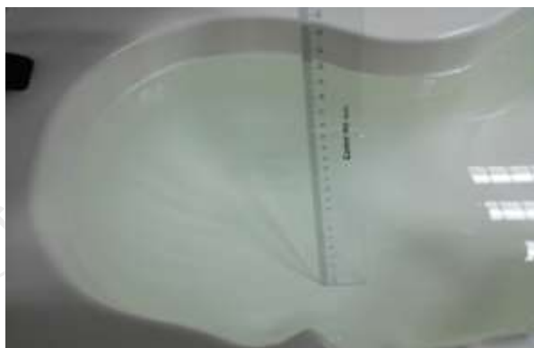
The Head Liquid of 2450MHz (15.6cm)
