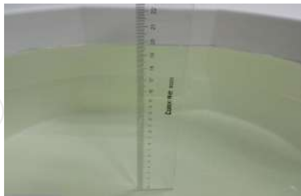
The Body Liquid of 835MHz (15.4cm)
