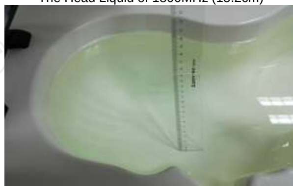
The Head Liquid of 750MHz (15.3cm)
