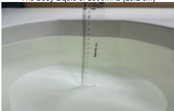
The Body Liquid of 2450MHz (15.3cm)
