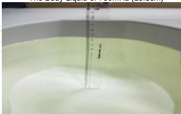
The Body Liquid of 1800MHz (15.2 cm)
