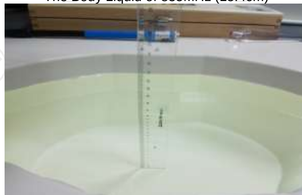
The Body Liquid of 1900MHz (16.4 cm)
