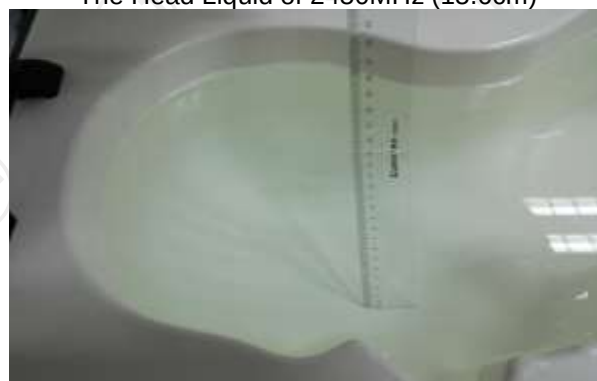
The Head Liquid of 1800MHz (15.2cm)
