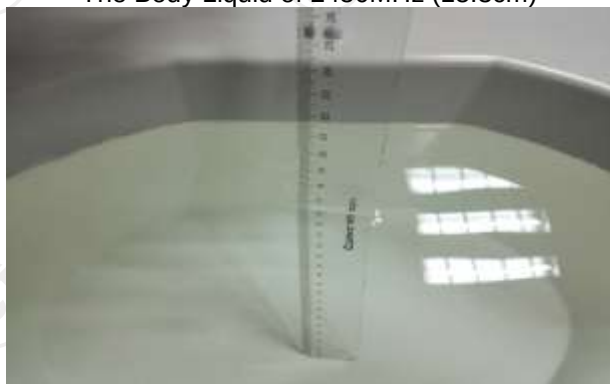
The Body Liquid of 5000-6000MHz (16.5cm)
