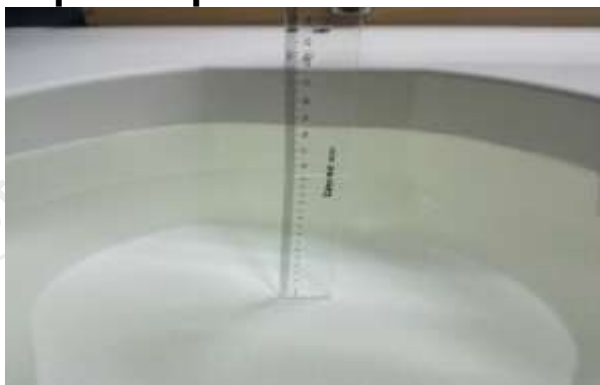
The Body Liquid of 750MHz (15.3cm)
