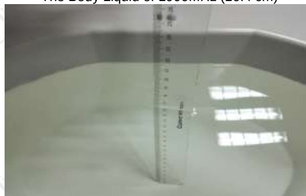
The Body Liquid of 2600MHz (16.5cm)
