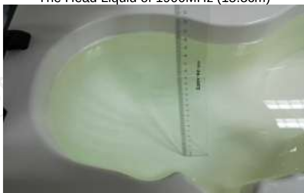
The Head Liquid of 835MHz (15.3cm)
