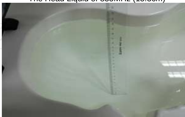
The Head Liquid of 2600MHz (15.1cm)
