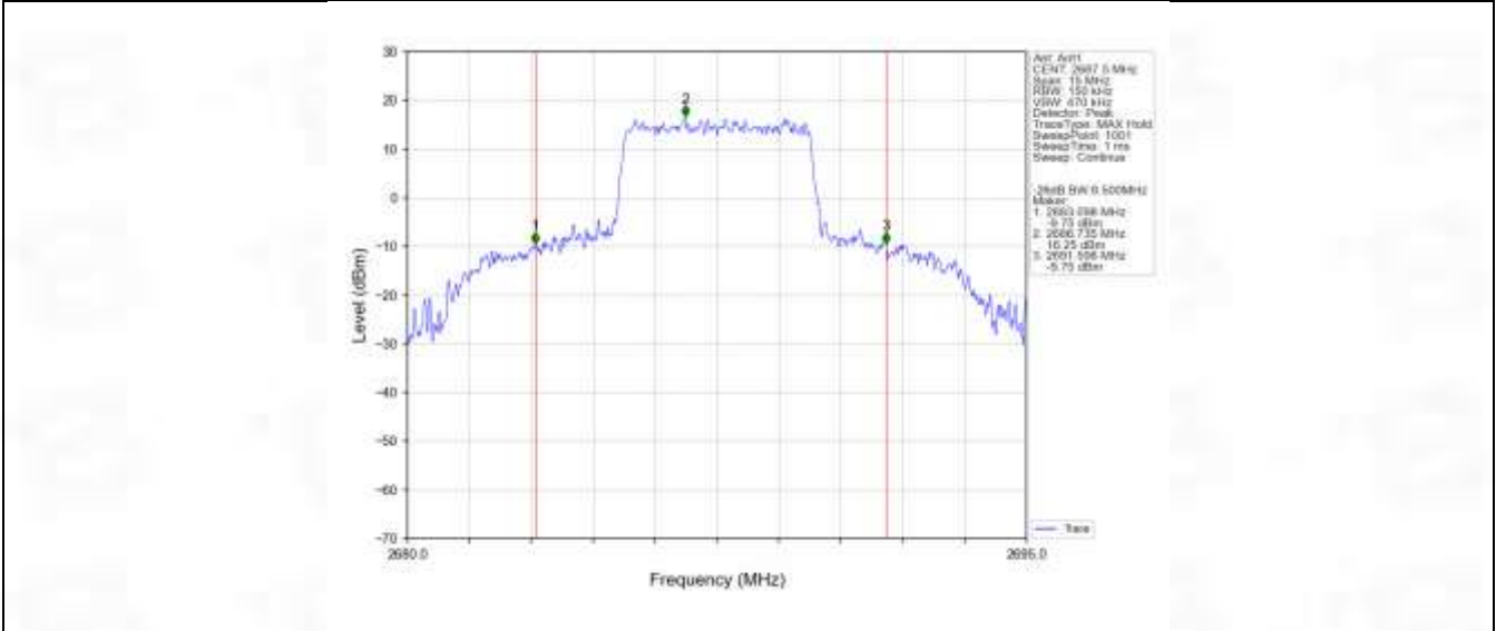
Band41 5MHz 16QAM HCH 2687.5MHz RB 25 0 NTNV
