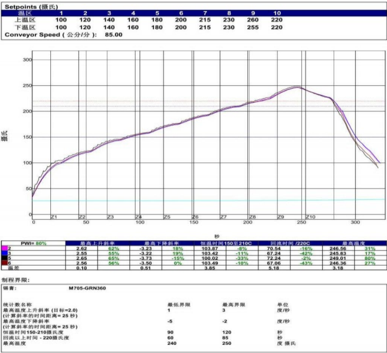
Figure 38 Temperature Curve of Solder Reflow
