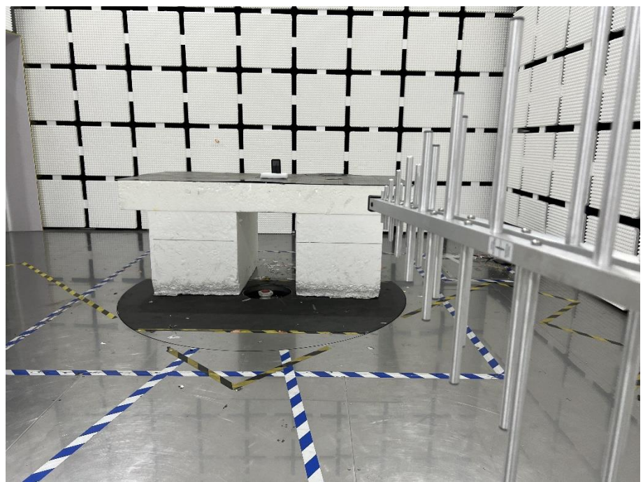
Radiation Emission Test Setup (30MHz to 1GHz)
