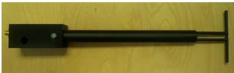
Figure 1 – MVG COMOSAR Validation Dipole
