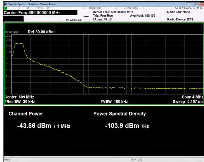
Band71 QPSK BW=15MHz Channel=133397 RB Size=1 Position=#Max Normal
