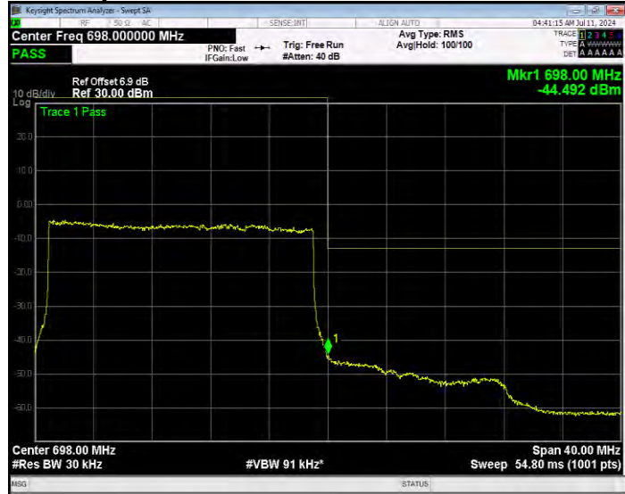
Band71 QPSK BW=5MHz Channel=133147 RB Size=1 Position=#0 Extended
