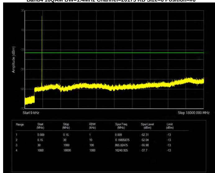
Band4 16QAM BW=1.4MHz Channel=20393 RB Size=6 Position=#0
