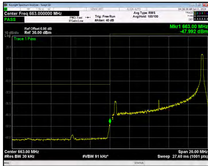
Band71 16QAM BW=10MHz Channel=133172 RB Size=50 Position=#0 Extended
