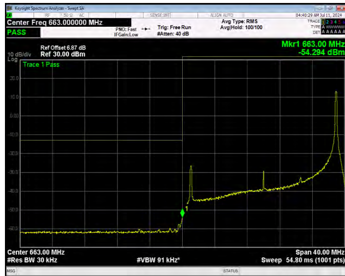
Band71 16QAM BW=20MHz Channel=133222 RB Size=100 Position=#0 Extended
