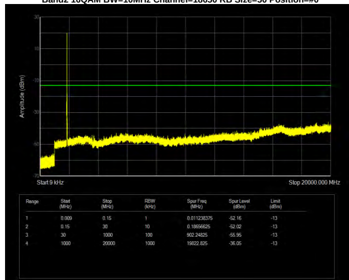
Band2 16QAM BW=10MHz Channel=18900 RB Size=50 Position=#0
