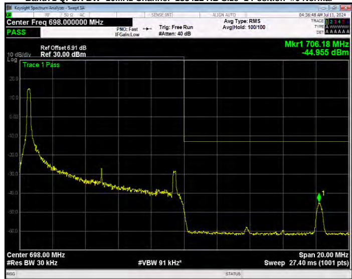
Band71 QPSK BW=10MHz Channel=133422 RB Size=1 Position=#Max Extended
