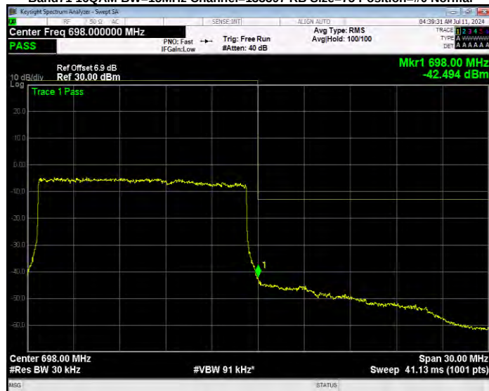
Band71 16QAM BW=20MHz Channel=133222 RB Size=1 Position=#0 Extended
