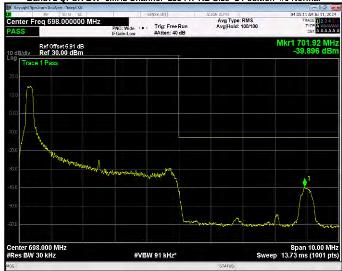
Band71 QPSK BW=5MHz Channel=133447 RB Size=1 Position=#Max Extended
