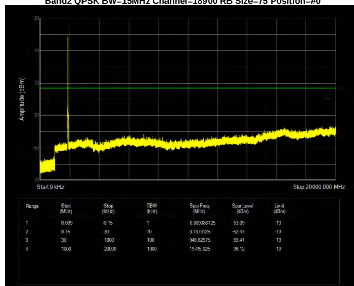
Band2 QPSK BW=15MHz Channel=19125 RB Size=75 Position=#0
