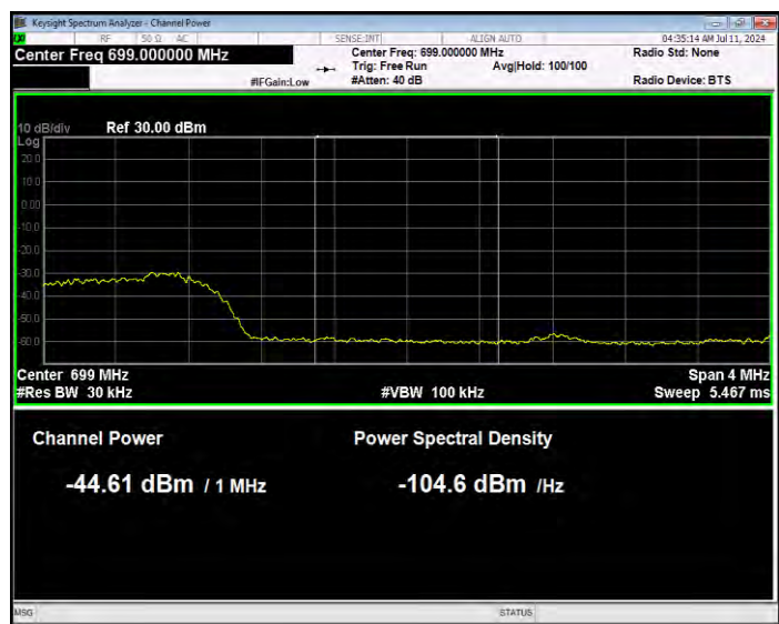
Band71 QPSK BW=5MHz Channel=133447 RB Size=1 Position=#0 Normal
