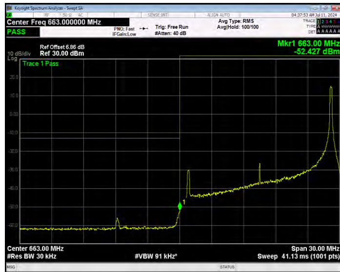
Band71 QPSK BW=15MHz Channel=133197 RB Size=75 Position=#0 Extended
