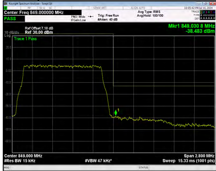
Band5 QPSK BW=10MHz Channel=20450 RB Size=1 Position=#0 Extended
