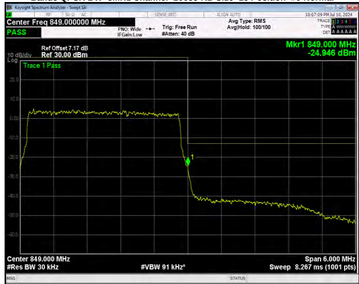
Band5 QPSK BW=5MHz Channel=20425 RB Size=1 Position=#0 Extended
