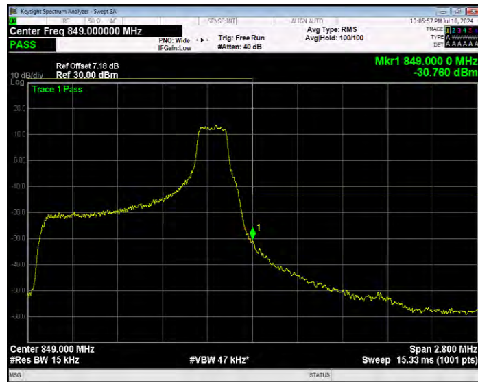
Band5 16QAM BW=1.4MHz Channel=20643 RB Size=6 Position=#0 Extended
