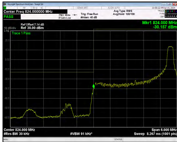
Band5 QPSK BW=3MHz Channel=20415 RB Size=15 Position=#0 Extended
