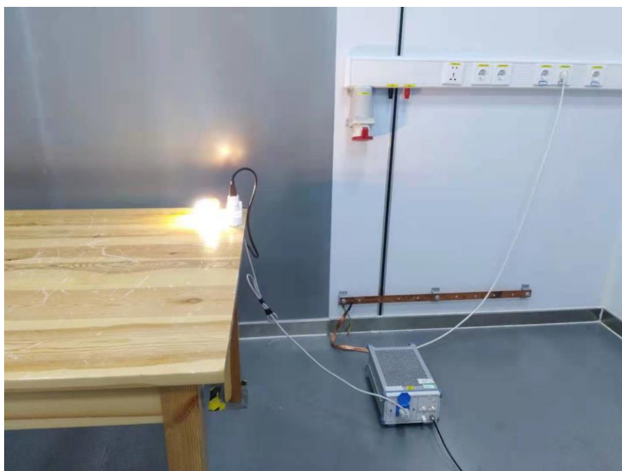
Fig. 4 Power line conducted emission setup photo
