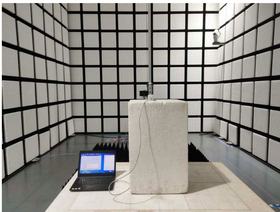
Fig. 3 Radiated emission setup photo(Above 1GHz)
