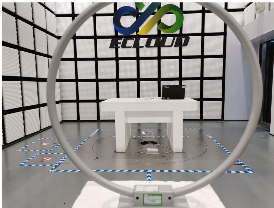
Fig. 1 Radiated emission setup photo(Below 30MHz)
