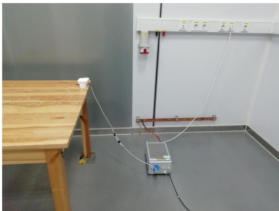
Fig. 4 Power line conducted emission setup photo
