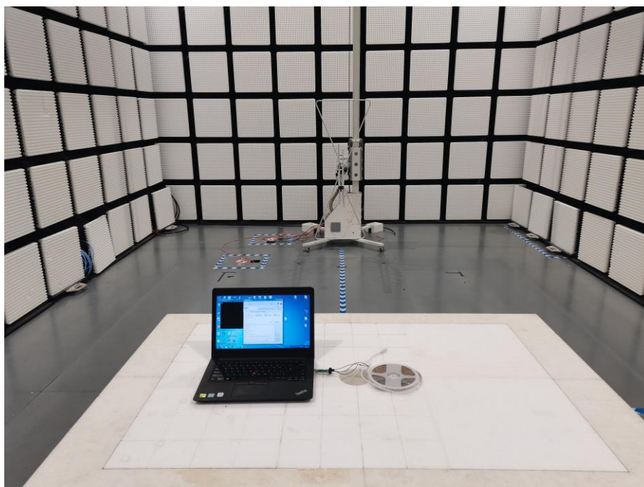
Fig. 2 Radiated emission setup photo(30MHz-1GHz)
