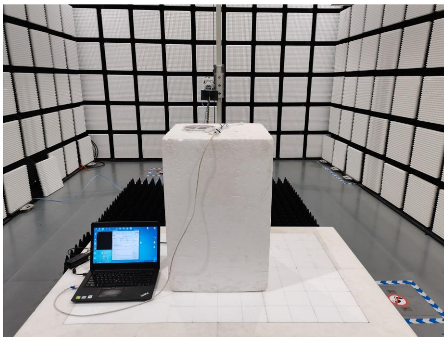
Fig. 3 Radiated emission setup photo(Above 1GHz)
