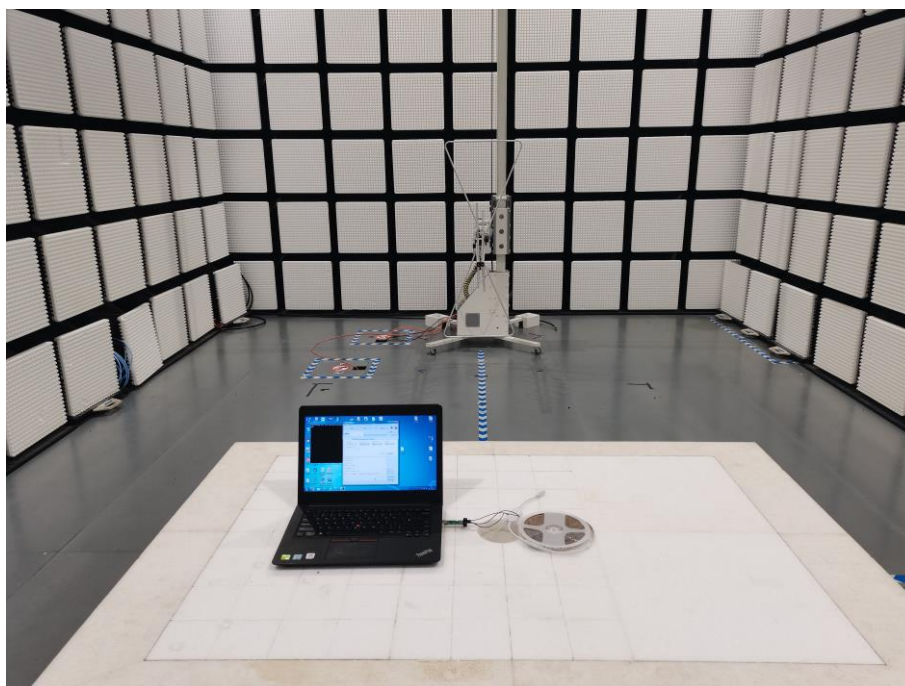
Fig. 2 Radiated emission setup photo(30MHz-1GHz)
