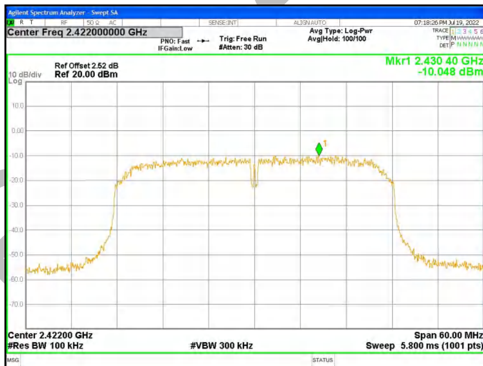
Band Edge NVNT n40 2422MHz Ant1 Emission
