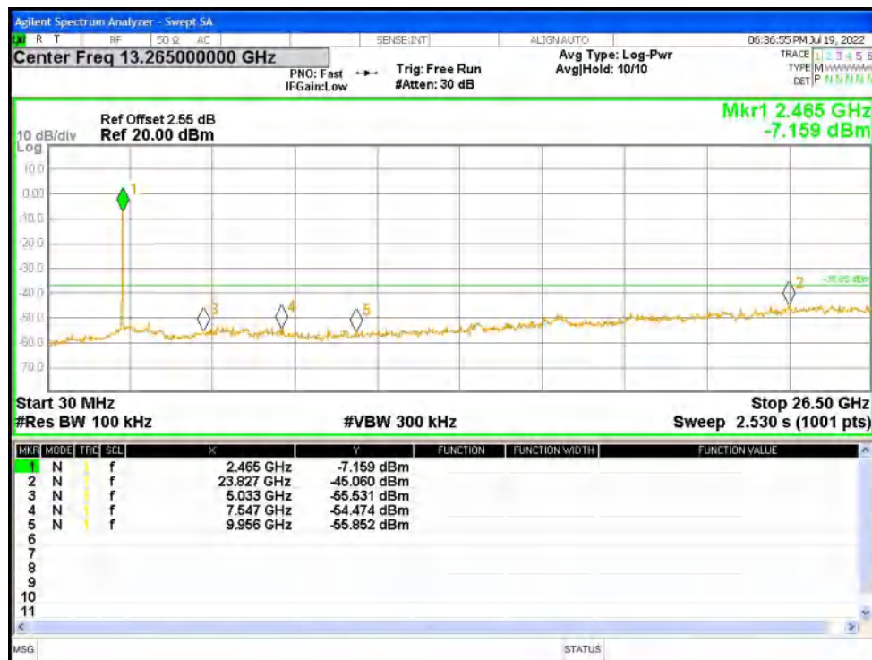
Tx. Spurious NVNT n20 2412MHz Ant1 Ref
