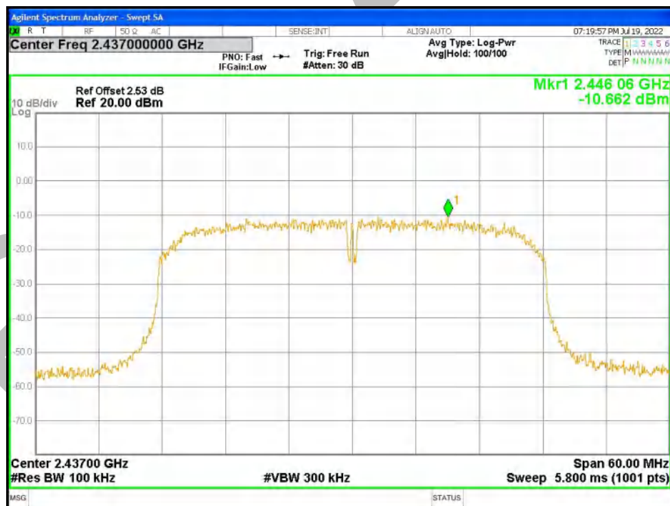
Tx. Spurious NVNT n40 2437MHz Ant1 Emission
