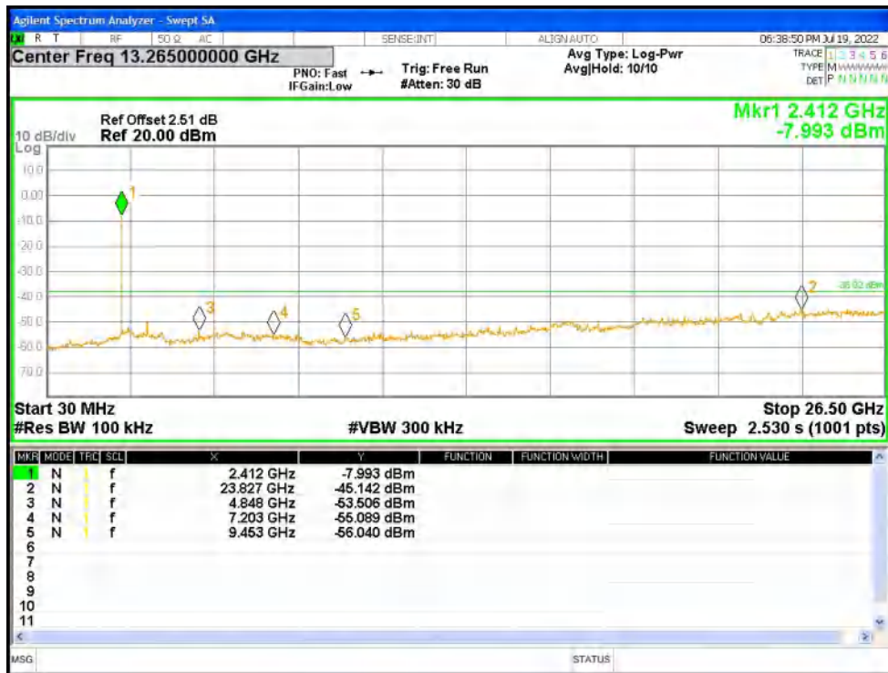
Tx. Spurious NVNT n20 2437MHz Ant1 Ref
