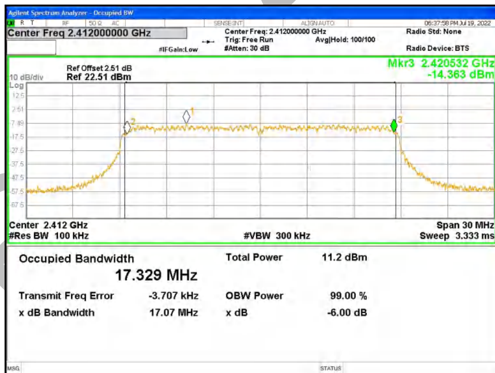
-6dB Bandwidth NVNT n20 2437MHz Ant1
