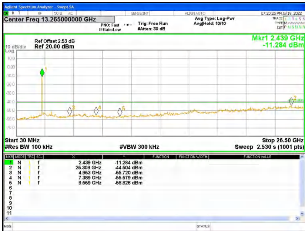
Tx. Spurious NVNT n40 2452MHz Ant1 Ref
