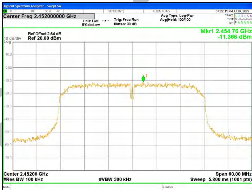
Band Edge NVNT n40 2452MHz Ant1 Emission
